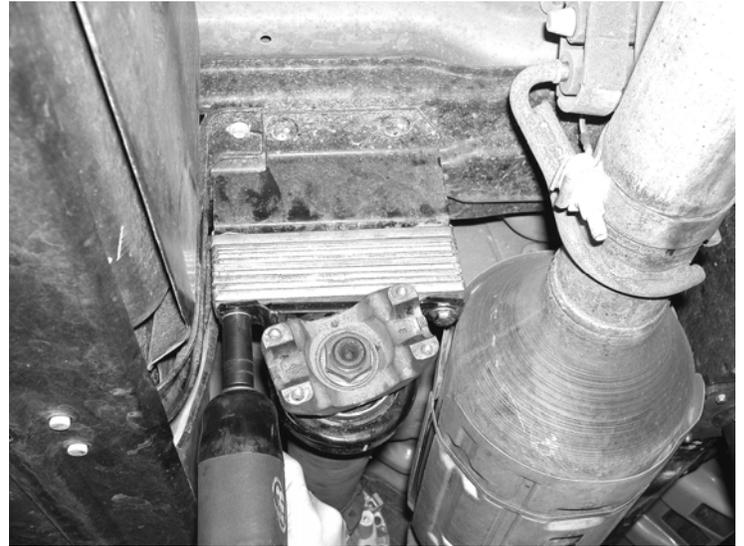
11. Re-align marks on front and rear drive shaft halves and re-attach with factory hardware. SEE PHOTOS BELOW.
