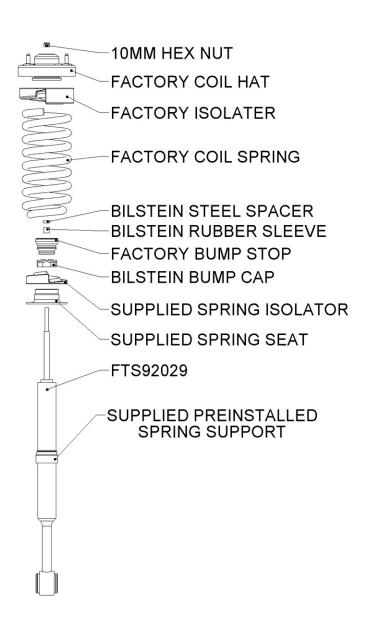
4. Reinstall the new coil over assembly into the upper mount and the lower control arm mount. Torque the upper 3 nuts to 35 ft-lbs and the lower bolt to 110 ft-lbs. SEE PHOTO BELOW.
