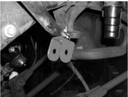
3. Locate the new Fabtech lower sway bar end link bracket FT50036. Attach to the factory axle mount with the supplied ½" x 1 ½" bolt, nut and washer. Note: there is a driver and passenger side bracket, when installing the bracket make sure the key way on the bracket is locked into the factory mount and the new bracket is straight up and down. SEE PHOTO BELOW.
