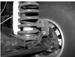
4. Locate the new Fabtech sway bar end link FT50070. Install one hour glass bushing and one ½" sleeve into each end of the new Fabtech sway bar end link With the supplied ½" x 2 ¾" nut, bolt, and washers connect to the upper sway bar mount. Note: when installing the sway bar end links, make sure the tab on the end link is facing back on the upper inboard side. SEE DRAWING BELOW.
