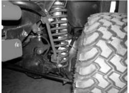
9. Recheck all nut and bolts for proper torque tightness before driving.
