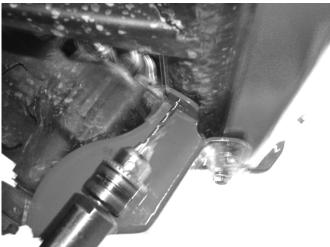
8. Torque the steering box bolt to 70 Ft. Lbs. Torque the bumper bolt to 80 Ft Lbs. Torque the inner bolt 30 Ft. Lbs.
