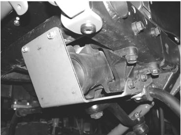
5. Tighten Up steering box bolts torque to 70 Ft. lbs.
