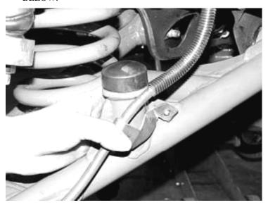
14. Remove the factory tie rod adjuster sleeve and install the new extended adjusters. One side of the adjuster is threaded left hand and one is right, be sure to use the proper side on each tie rod end. Thread both tie rods in until they completely bottom out. Connect the tie rod end to the spindle and reinstall the original castle nut. Fully tighten the castle nut and install a new cotter pin. Rotate the adjuster sleeve out to set a rough toe in. SEE PHOTOS ON NEXT PAGE.
