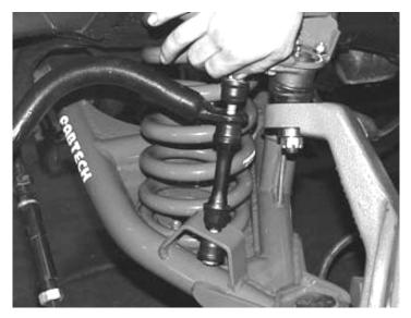
17. The ABS sensor line needs to be routed inside the UCA, then down to the spindle. Secure the ABS line to the inside of the UCA tube where it cannot come into contact with the tire in full right or left hand turns.
