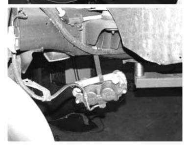
4. Support the LCA with a floor jack and compress the suspension ½" to ½". Remove the castle nuts securing the upper and lower ball joints to the spindle. Separate the ball joints from the spindle and set the spindle aside. Lower the jack supporting the LCA and remove the coil spring from the truck. Keep the upper coil spring insulators. Remove the 2 LCA pivot bolts and set the LCA aside. SEE PHOTOS BELOW.
