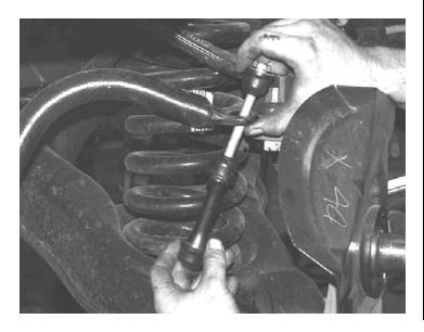
3. Starting on the driver's side of the truck, support the lower control arm (LCA) with a jack. Remove the cotter pin and castle nut attaching the tie rod end to the spindle. Separate the tie rod end from the spindle. Remove the brake line support tab from the LCA. Remove the two bolts securing the brake caliper to the spindle. Tie the brake caliper up and out of the way. DO NOT LET THE BRAKE CALIPER HANG FROM THE BRAKE LINE. SEE PHOTOS ON NEXT PAGE.
