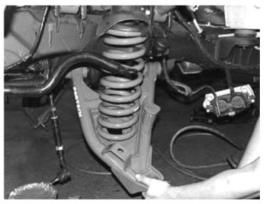
12. Reinstall the spindle onto the ball joints. Place the supplied 3/8" thick spacer on the upper ball joint before installing the castle nut and fully torque both castle nuts and install two of the newly supplied cotter pins. Release the floor jack supporting the lower control arm. If you are installing this kit with stock spindles use the 2" tall bump stops or if you are installing this kit with 3" Fabtech lift spindles use the 1" tall lower bump stop in the LCA. SEE PHOTOS IN NEXT COLUMN.
