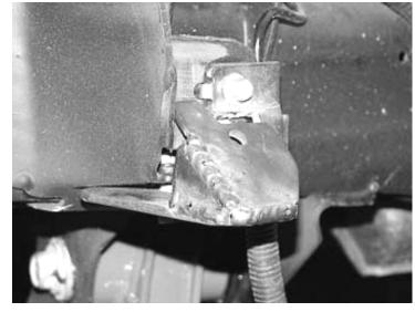
7. Using a MIG welder, weld the top of the bump stop bracket line bracket to the frame mount. Once the parts have fully cooled, paint all exposed metal surfaces. Install a 1" tall urethane bump stop into the mount. SEE PHOTOS BELOW.
