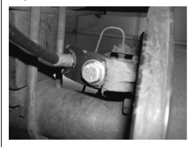
20. Locate the factory brake line mount on the driver side of the axel. Remove the vent line from the bolt and remove bolt, save hardware. Locate the supplied brake line bracket FT30042, attach the side with the sleeve to the axel using the factory hardware. Using the supplied 3/8" x 1 3/4" bolt, nut, and washer attach the brake line to the other end. Reattach vent line. SEE PHOTO ON NEXT PAGE. (This bracket will only be used on pick-up trucks).
