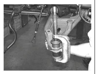
10. Press four FT1001 urethane bushings into the driver's side UCA followed by two sleeves. Be sure to thoroughly lubricate all bushings and sleeves with the supplied silicon lube. IF YOUR TRUCK DOES NOT HAVE THE ADJUSTABLE "D" BOLTS AND WASHERS ON THE UPPER CONTROL ARM MOUNTS, YOU WILL NEED TO PURCHASE A FTS290 KIT FROM FABTECH. THE FTS290 KIT INCLUDES BOLTS AND WASHERS WHICH ALLOW FULL ALIGNMENT ADJUSTMENT.
