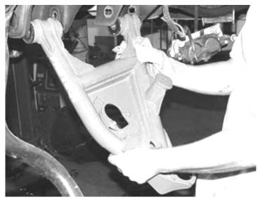
9. Using a ball joint press, remove the original lower ball joint from the factory LCA and press it into the new LCA, in the same direction it was removed. SEE PHOTO BELOW
