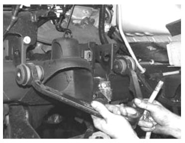
6. Using a die grinder with a cutoff wheel, notch the brake line tab as shown on the bump stop frame mount. Remove the original lower bump stop from the frame mount and install the bump stop bracket using the original bolt without the original lower bump stop. SEE PHOTOS BELOW.
