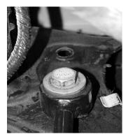
10. Thread the urethane bump stops onto the bump stop extensions. Using a drill, drill the original hole open to 7/16", attach the bump stop extensions to the differential pad using the supplied 7/16 x 1 ½" bolts and nut tab FT90038, along with a small amount of the supplied thread locking compound, (the nut tab will be inserted from the front side of the axle) and torque to 35lbs. Make sure you align the locator pin in the extension with the hole in the axle pad.
