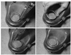
Remove the snap ring from the top of the lower ball joint. Place one FT97159-7-101 shim over the ball joint and replace the snap ring on the lower ball joint, making sure the snap ring is fully seated in the groove.
