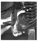
7. Use a ball joint puller to separate the spindle from the ball joints and set the spindle assembly aside.
