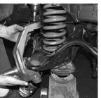
9. Take the passenger's side lift spindle and slide it onto the upper and lower ball joints. Reinstall the original castle nuts. Torque the castle nuts to factory
