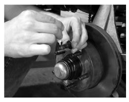
11. Place the tie rod end into the spindle. Reinstall the castle nut and torque it to 35 ft-lbs. Aligning it with one of the cotter pin holes in the tie rod end. Install one of the new supplied cotter pins. SEE PHOTOS BELOW.
