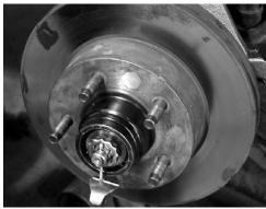
10. Slide the brake caliper back onto the spindle. Place several drops of thread locking compound onto the original lower brake caliper bolt and attach the caliper to the spindle. Use one of the supplied 12mm-1.75 x 70mm bolts in place of the original upper caliper bolt with thread locking compound. Torque the bolts to 35 ft-lbs. SEE PHOTO BELOW AND IN NEXT COLUMN.
