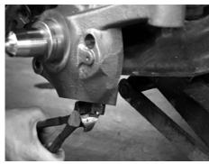
9. Grease the end of the spindle with high temperature brake grease and slide the rotor onto the spindle. You may want to repack the wheel bearings if the bearing grease shows any signs of aging or wear. Replace the original castle nut and tighten it just enough to remove any bearing play in the rotor, make sure the rotor can spin freely. Place the cotter pin locator onto the spindle and install one of the new supplied cotter pins. SEE PHOTOS BELOW.
