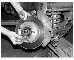
4. If this truck is equipped with front ABS, separate the line from the spindle and set the sensor aside. Remove the top clinch bolt from the spindle. Remove the cotter pin and castle nut from the lower ball joint. Separate the lower ball joint from the spindle and slide the spindle off the ball joints. SEE PHOTOS BELOW.
