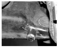
7. On models with front ABS, attach the sensor to the spindle in the provided hole. Use a ¼" x 1-¾" bolt, ¼" lock washer and ¼" flat washer to mount the sensor. Use the ¼" x ¾" bolt, ½" lock washer and ¼" flat washer to attach the ABS sensor wire to the back of the spindle. SEE PHOTO BELOW AND IN NEXT COLUMN.
