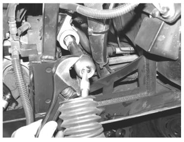
Locate FT95025 Driver Inner Tie Rod Bracket and the supplied 12mm bolt and thread-locking compound. Position the bracket to the rack & pinion and attach with the 12mm hardware. Use some of the supplied thread-locking compound and torque to 75 lbs. SEE PHOTOS BELOW.
