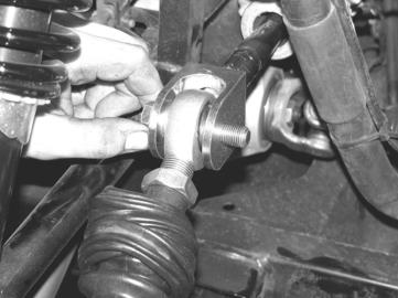
12. Locate FT95011 Heavy Duty Steering Arm Hat and install into the steering knuckle. Locate FTS43 Mis-alignments and the supplied ½" x 3 ½" hardware. Install the mis-alignments into the right hand thread heim and place on top of the steering hat. Inset the ½" bolt from the top of the heim and down into the knuckle. Place one ½" washer on the bottom of the knuckle with a C-Lock nut. Torque to 75 lbs. SEE PHOTOS BELOW
