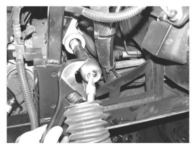
7. Locate FT95025 Driver Inner Tie Rod Bracket and the supplied 12mm bolt and thread-locking compound. Position the bracket to the rack & pinion and attach with the 12mm hardware. Use some of the supplied thread-locking compound and torque to 75 lbs. SEE PHOTOS BELOW
