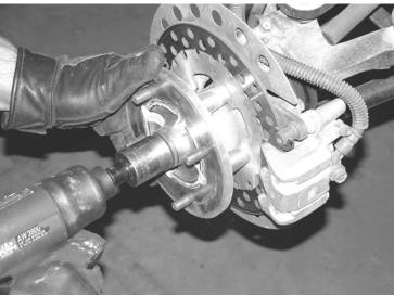
3. Remove the two 10mm bolts that attach the brake line to the spindle and the upper control arm and save the hardware. Remove the brake caliper and hang on the frame. DO NOT LET THE CALIPER HANG BY THE BRAKE HOSE. Remove the rotor and hub assembly and save. Remove the brake rotor shield from the spindle and save with the hardware. SEE PHOTOS IN NEXT COLUMN
