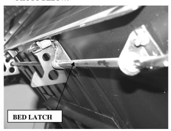
2. Support the bed in up right position. Locate bed struts and hardware. Remove the (2) bolts at the top of strut on the mount. Now remove the nut off the lower mounting point and discard struts and hardware. **SEE PHOTO BELOW.**
