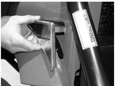
5. From the inside of the bed reinstall the factory tie down loop with the factory nuts. Torque the nuts to 15 foot lbs. **SEE PHOTO ON NEXT PAGE.**
