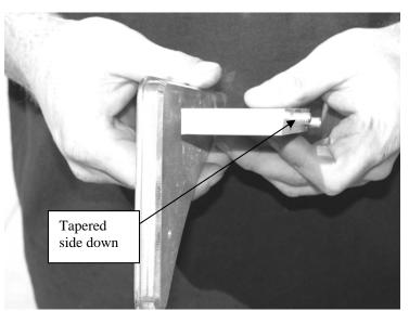
4. Install the cover into the pocket were the bed tilt leaver use to be located. Using the two factory holes slide the all thread through. **SEE PHOTO BELOW.**
