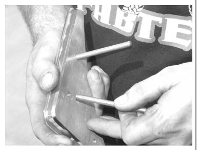
2. From the inside of the bed remove the two cap nuts holding the tie down loop on and remove the factory bolts. Discard the bolts saving the factory cap nuts.
