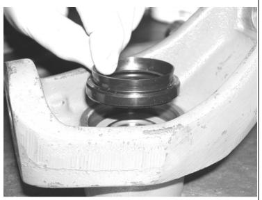
**10.** Reinstall the spacer and outer bearing using the method as on the inner bearing. SEE PHOTOS BELOW AND IN NEXT COLUMN.
