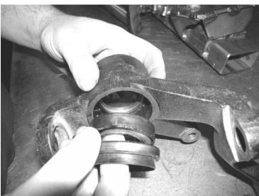
**8.**Locate FT95159D and FT95159P. Apply grease to the bearing surfaces of the spindle. Start with the inner bearing and Tap evenly in to the new spindle using a large socket or piece of tubing that fits the outside of the bearing and inside of the spindle. SEE PHOTOS BELOW AND ON NEXT PAGE.
