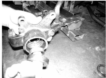
**7.** Flip the spindle over and tap out the inner bearing this will push the seal at the same time. These will be reused in the new spindle. SEE PHOTOS IN NEXT COLUMN.
