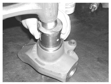
**11.** Reinstall the outer being seal careful not damage it. SEE PHOTO BELOW.
