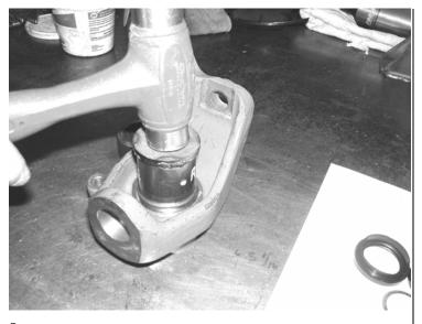
**9.** Reinstall the inner bearing seal that has the tall lip for the C.V. to sit in. Careful not to damage. SEE PHOTO BELOW.
