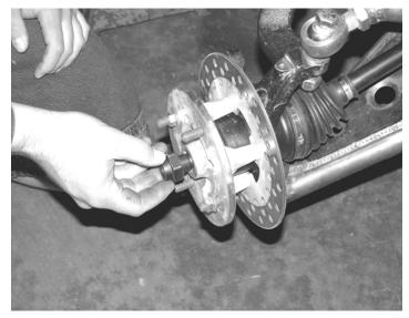
8. Locate the 10mm brake caliper bolts and re-attach the rotor. Torque to 35 ft. lbs. (use supplied thread-locking compound) Locate the two of the supplied adel clamps and ¼" hardware. Position the adel clamps over the brake hose and attach to the tabs on the upper control arms. Torque to 10 lbs. SEE PHOTO BELOW.
