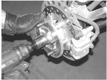
3. Remove the two 10mm bolts that attach the brake line to the spindle and the upper control arm and save the hardware. Remove the brake caliper and hang on the frame. DO NOT LET THE CALIPER HANG BY THE BRAKE HOSE.
