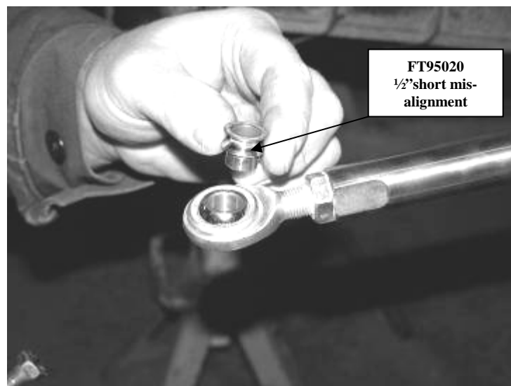
New Tie Rod Assembly @ Knuckle
