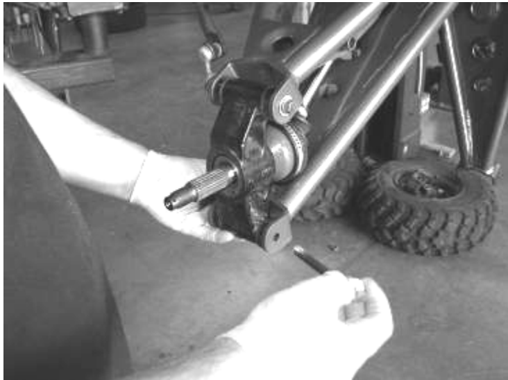
60. Attach factory knuckle to lower control arm with factory hardware. Leave loose. SEE PHOTOS BELOW.
