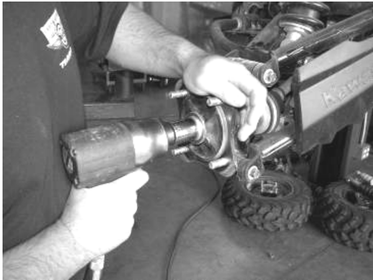
46. Remove the upper and lower knuckle hardware and remove the knuckle. Save the knuckle and the hardware. SEE PHOTOS BELOW AND ON NEXT PAGE.
