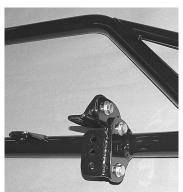
1. Disconnect the negative terminal on the battery. Using the supplied 3/8" hardware, attach the 2 mounting brackets to the new bumper. There should be a 3/8" flat washer on each side of the bolt. Leave the bolts loose enough to allow adjustments in the bracket positions. Repeat this on the opposite side of the bumper.
