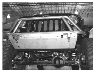
4. Using the Two holes in the bottom corners of the Skid Plate as a template drill out the two 5/16" holes in the bottom corners and insert the supplied 5/16" hardware. Torque to 20 Ft Lbs. SEE PHOTOS IN NEXT COLUMN.
