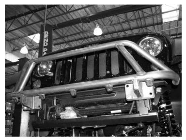
3. Locate the Fabtech Skid Plate FT50364BK. Using the supplied 5/16"x 1" bolts, flat washers, and split washer attach the top of the skid plate to the bumper. You will want the flat washer against the skid plate. Torque to 20 Ft Lbs. SEE PHOTO BELOW.
