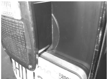
7. Re-install the taillight housings, license plate and holder, and gas filler pocket using the factory hardware. SEE PHOTO BELOW.
