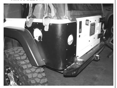
3. A 7/32" pilot hole must be drilled prior to installing the new bolts. Start with the front lower mounting hole. Make sure that there is no wiring other items that will be damaged while drilling. SEE PHOTO BELOW.
