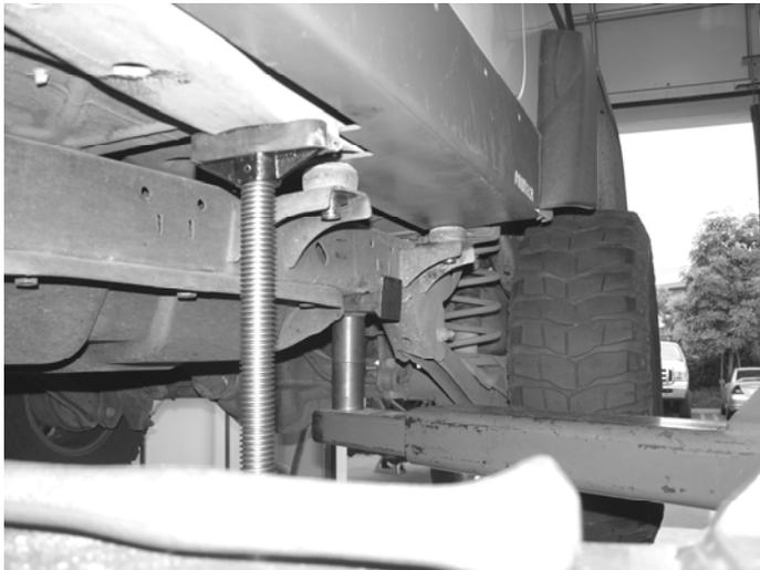
3. The factory body bushing will need to be cut to allow the Rocker Guard to be mounted between the body mounts and the cab of the Jeep. Measure, mark, and cut 3/16" from the top of the bushing. Replace the body bushing and hardware back onto the Jeep leaving the hardware loose SEE PHOTO BELOW AND IN NEXT COLUMN.
