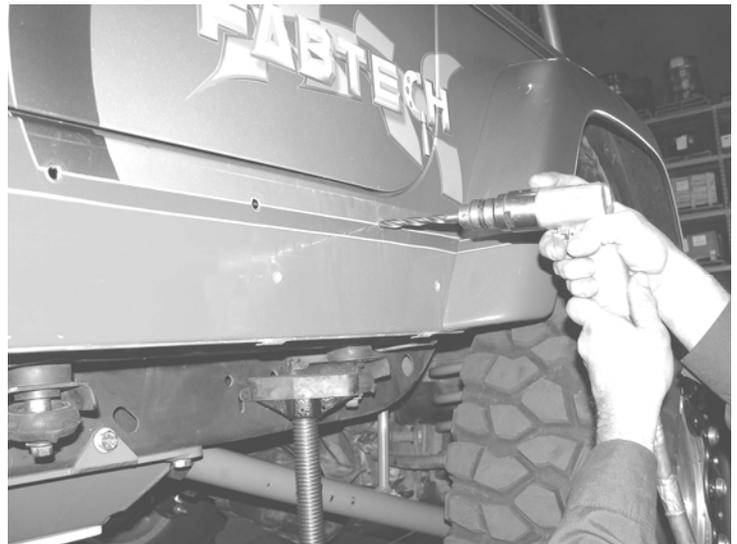
6. Clean all of the metal shavings from drilling off of the body. Use paint or clear silicone to cover any raw or
