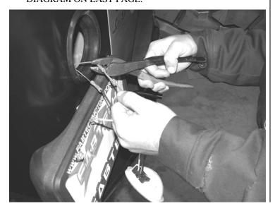
4. Test the Brake, Turn Signals, and the Running Lights to make sure that all your connections are good and working properly before installing the new lights. Tape up the unsed reverse and license plate wires, DO NOT LEAVE EXPOSED. Then insert the new L.E.D. into the Rubber Ring that is in the Jeep. SEE PHOTOS BELOW.
