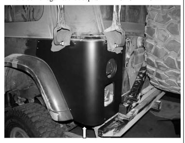
3. Using a drill with a 7/32" drill bit, drill the pilot holes for the mounting bolts. Start with the front lower mounting hole. Make sure that there is no wiring other items that will be damaged while drilling. SEE PHOTO BELOW.
