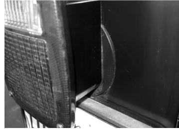
7. Attach the factory gas filler tube to the factory gas filler pocket using the factory hardware. Use the supplied 10/32" thread forming bolts, attach the license plate and holder, and gas filler pocket to the body. NOTE- These are thread forming bolts, use care when installing them, DO NOT OVER TIGHTEN THEM.
