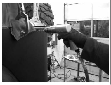
4. Install the supplied Counter-sunk Torx bolts. Install the nylock nuts, and washers to ALL EXPOSED BOLTS ON THE INSIDE OF THE JEEP. The self-threading bolts are ONLY to be used WITHOUT the nylock nuts where there is no access to the backside of the bolt. Do not over tighten the bolts where a nylock will not be used. SEE PHOTOS BELOW.
