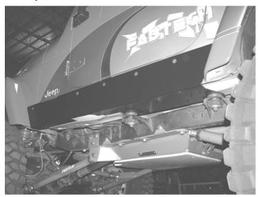
7. If your Jeep has the fender flares that run along the body, you will need to trim the bottom of the flare for proper clearance of the flare to the rocker guard. Mark and cut the flare as desired. SEE PHOTOS ON NEXT PAGE.
